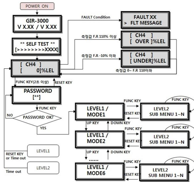
[Figure 16. Configuration of GIR-3000 mode]
