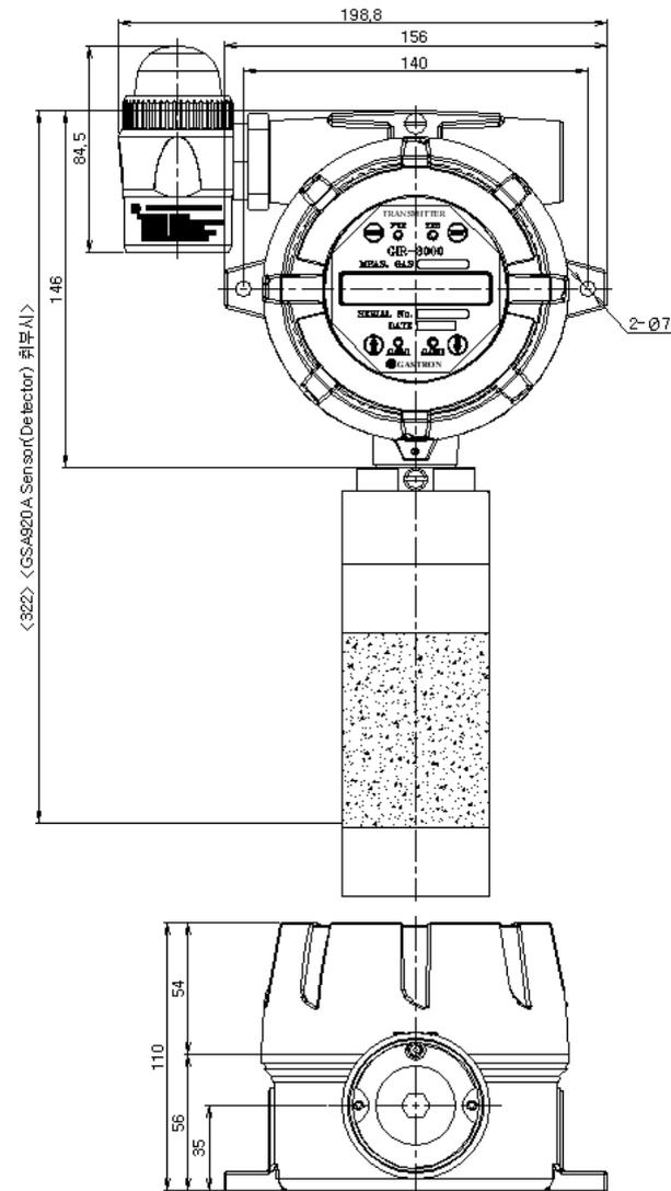
[Figure 18. Outline drawing for coupling of GIR-3000 warning light]
