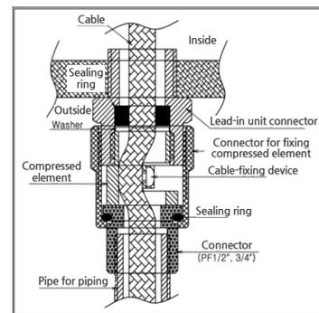
[Figure 21. Pressure-resistant packing type]
