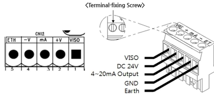
[Figure 6. Configuration of CN12 terminal]
