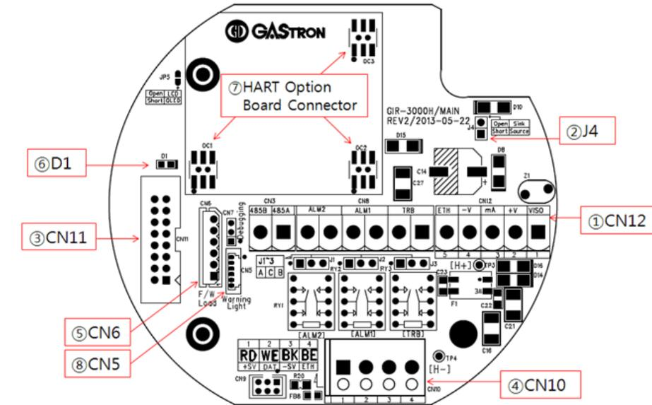
[Figure 5. Layout diagram for Main PCB terminals]
